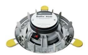
To benefit installers, Russound developed spring-clip locking retainers that reduce installation time. In-ceiling speakers are simply pressed into the cutout, enabling the clips to snap into place and secure the speaker. For the in-wall model, the spring clips hold the speaker in the wall, making it easier to square up the speaker while tightening the dogleg grips.
