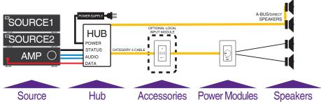
Figure 2: Basic Custom Home A-BUS System Architecture
