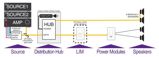
Figure 3: Basic Structured Wiring A-BUS System Architecture
