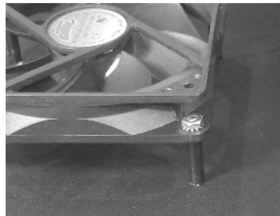
Figure 2 – Shelf mode fan mounting
